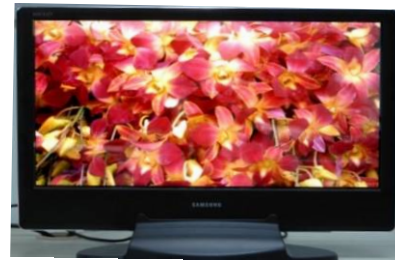
19" qFHD (FPD2009) Oxide TFT (The first)
