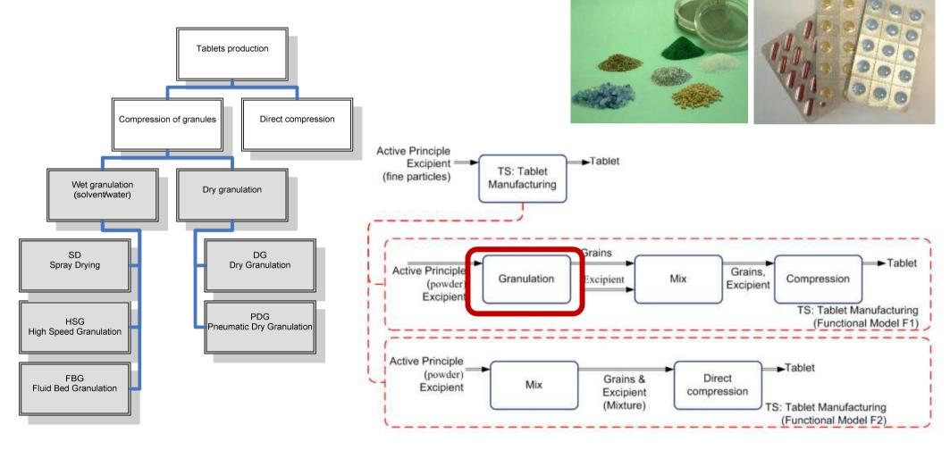
Behavioral Models associated to the elementary functions of alternative granulation technologies
