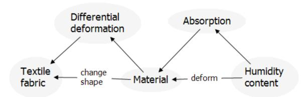
**43.** A textile fabric including a material adapted to expand and/or contract in response to a change in relative humidity and/or exposure to liquid sweat, the material being arranged in the fabric such that expansion and/or contraction of the material results in a change in one or more properties of the fabric, for example three dimensional geometry, insulation performance, air movement and/or liquid management.
