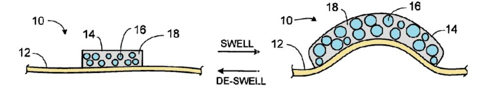
• A textile fabric (10) includes a smooth surface (12) with one or more regions having a bound coating of hydrogel (14) exhibiting expansion or contraction in response to change in relative humidity or exposure to liquid sweat or a combination thereof, adjusting insulation performance, air movement, and/or liquid management of the textile fabric 10) in response to ambient conditions.
