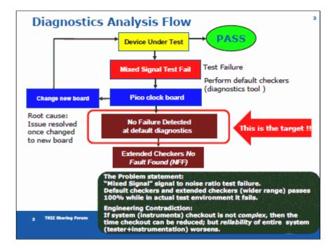
'The Solution – In order to understand further the nature of the problem, we simulated the problem in a controlled DOE (make it worst). Based on these findings a complete CEC and FUNCTIONAL DIAGRAM were developed to understand and define the interactions of the components.' [\*\*\* See the Functional diagram quoted earlier in this review.]
