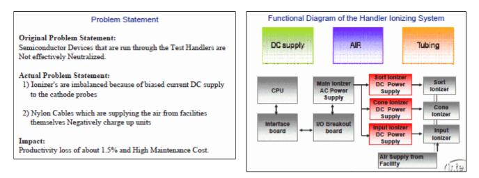
Thus, at the step of Trimming, it was natural to think of the trimming of the three sets of ionizers with individual power supplies into one set. The solution idea is shown below in the initial form of overview (below-left), and in the final form of concepts actually adopted (below-right).
