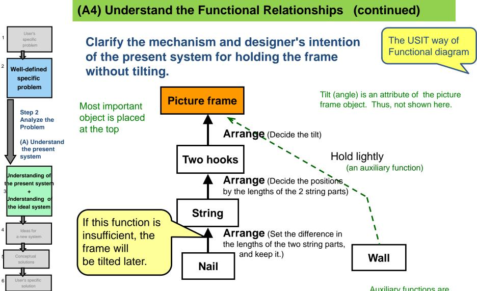
Harmful or insufficient functions may be commented explicitly, if significant. Auxiliary functions are drawn in broken lines.
