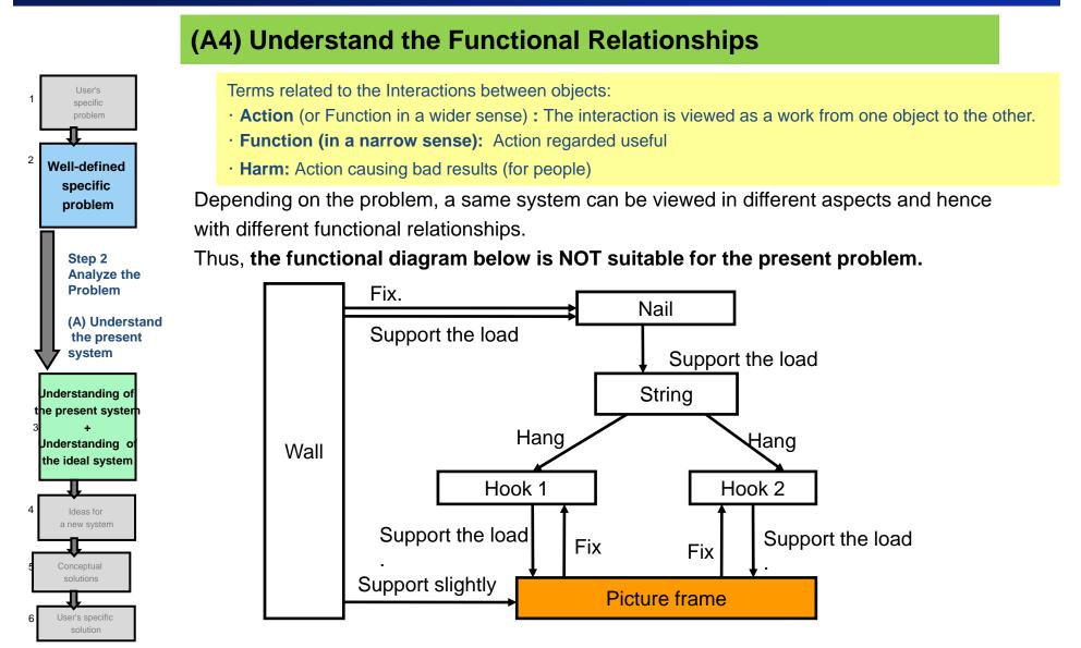
On the arrangement/tilt of the picture frame (and its adjustment and holding), no information is available in this diagram.
